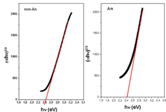
**Figure (6):The relationship between  $(\alpha h\nu)^2$  and photon energy for both annealed and non-annealed)  $V_2O_5$  thin films (red lines in both graphs represent the best intercept).**
