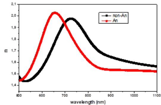
**Figure(3)The relationship between reflective index and wavelength for both annealed (red curve) and non-annealed (black curve)  $V_2O_5$ thin films.**
