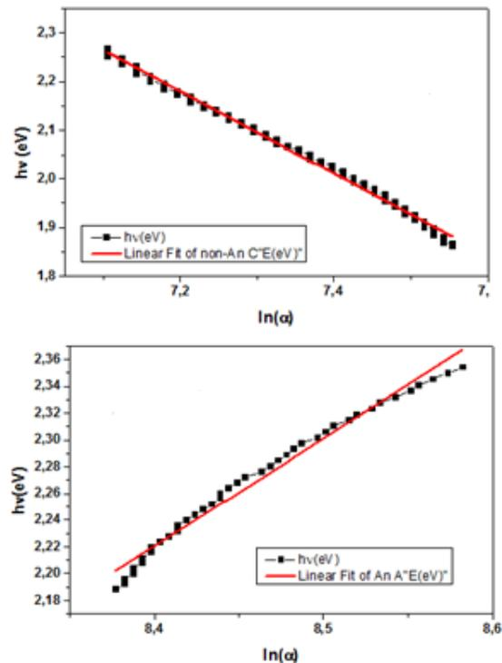
Figure(7): Variation of  $\ln\alpha$  and photon energy for both  $V_2O_5$  thin films (red lines are the best linear fit)
