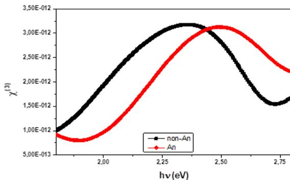
**Figure(5): Variations of the third order nonlinear optical susceptibility and photon energy for both annealed (red curve) and non-annealed (black curve)  $V_2O_5$  thin films.**
