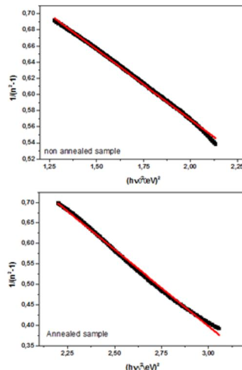
**Figure(4):The relationship between  $1/(n^2-1)$  and  $(h\nu)^2$  for both annealed (lower panel) and non-annealed (upper panel)  $V_2O_5$  thin films (red lines in both graphs represent the best linear fit). By plotting  $(n^2-1)^{-1}$  against  $(h\nu)^2$  and fitting a straight line as shown in Figure(4),**
