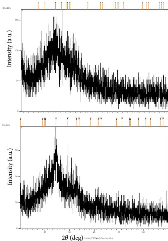
**Figure 2: XRD patterns for both non-annealed (upper panel) and annealed (lower panel)  $V_2O_5$  thin films.**
